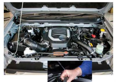
Heat and age are belts' and hoses' worst enemies. Other factors that hasten their demise include mileage, oil contamination, improper belt tension, failed hose clamps, or a burr or nick on a pulley.
